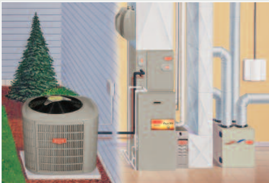
Air Conditioner and Gas Furnace System
