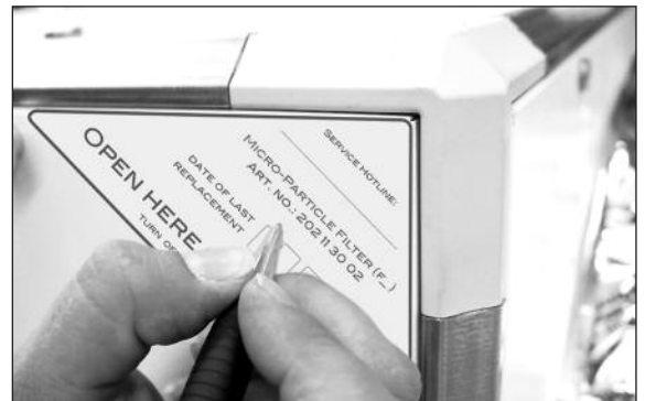
8. Fill out filter replacement label with scheduled date of next filter replacement. This should be no later than 3 years from current date, and affix on outer panel.
